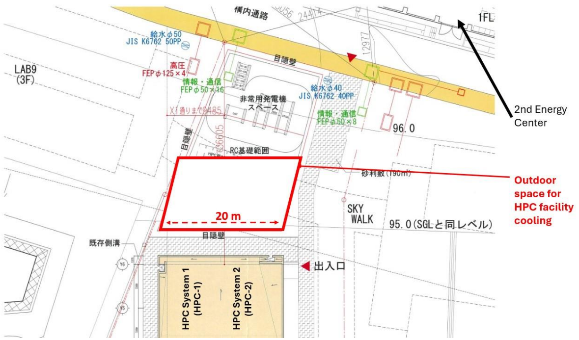
Fig. 7 Relative location of the room HPC-1 and the outdoor space (about 230 m 2 available) for the HPC facility cooling
