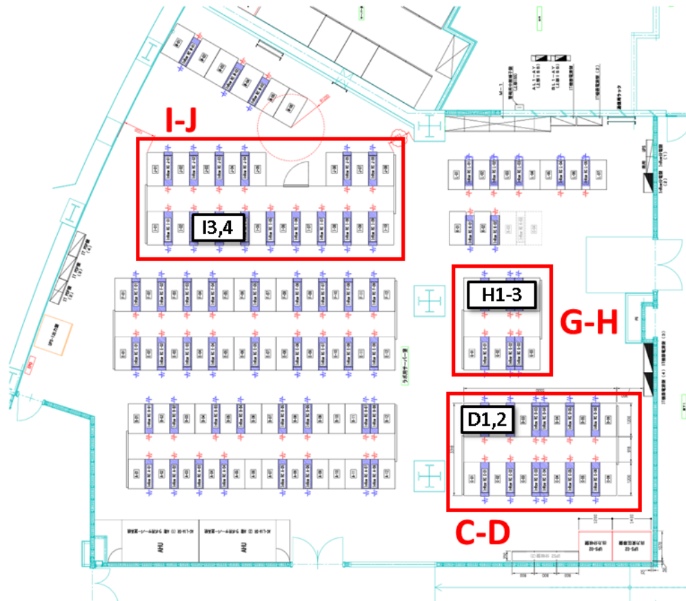
Fig. 2 Top view rack layout of OIST data center Lab1-A202 and location of existing storage system in racks D1-2, I3-4 and H1-3.
