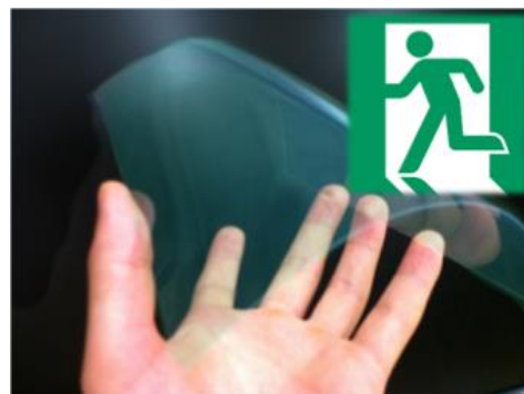
Figure 1. Flexible and transparent glow-in-the-dark film made by organic molecules.
