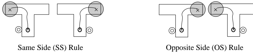
Figure 2: A schematic representation of the delayed response rules. Light samples are represented by double circles. Goal locations are represented by \times , while reward corresponds to the gray area. The behavioral task asks for controllers capable of switching between the two rules.
